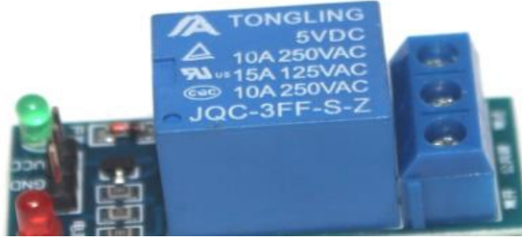
Figure 1: Single Channel Relay module
